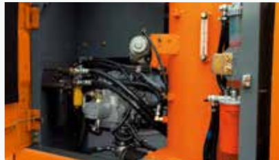
Grouped remote filters and inspection points
