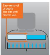
Parallel arrangement of radiator and oil cooler
