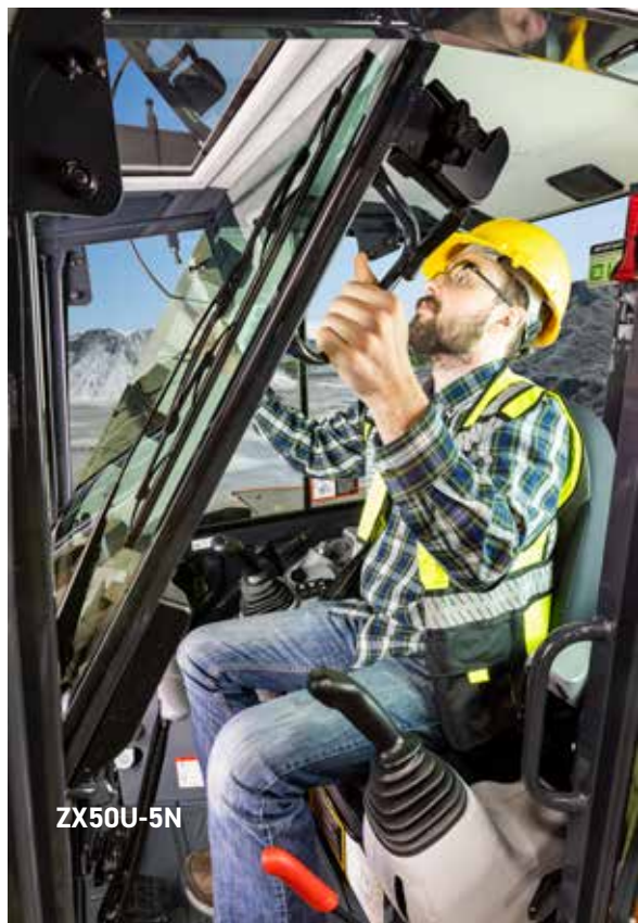
Above: Joystick controls for effortless operation and multi-function LCD eco-display makes operation easier.
