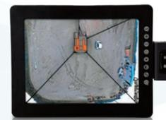
Aerial Angle provides the operator with a 360° view around their excavator. Cameras strategically mounted on the machine generate a single aerial view of the EX8000-7 surroundings. Multiple screen display options can be selected on the cab's 12-inch Aerial Angle monitor for ease of operation.
