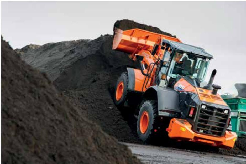
available in both auto and manual ranges, providing immediate access to extra rim-pull and breakout force for digging into heavy piles or for climbing grades with a full load onboard. Power Mode also provides a faster hydraulic speed to allow quicker bucket lifts, and does it all without limiting the loader's top speed. Power Mode lets you dig deeper, faster, and deliver more payload in every cycle.
