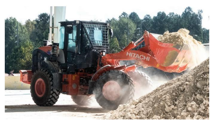
KaMin Performance Minerals bought the first Hitachi wheel loader sold in North America. This 141-horsepower ZW150-6 is used in the company's production of calcine from kaolin clay at their plant in Wrens, Georgia.
