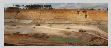
The kaolin is extracted from a mine about six miles from the KaMin processing facility. More than 100 feet of overburden, the brown material above the whitish-gray kaolin, must be removed to make the product accessible.
